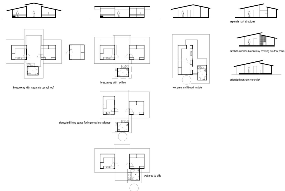
Figure 8: Options for the tjilpi house to balance indoor and sheltered outdoor living
